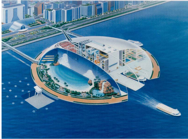
Fig. 1. A sewage treatment plant on a circular VLFS (Courtesy of the Floating Structures Association of Japan).
